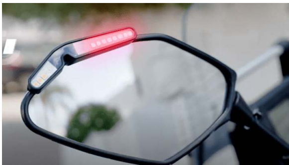
Fig 4. Top: common blind spot warning light integrated in a car mirror. Bottom: rare motorcycle add-on for a blind spot warning light.
