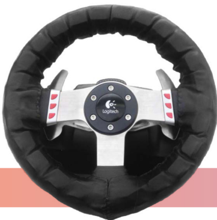
Fig 5. Prototype of a steering wheel with haptic (vibration) feedback.
